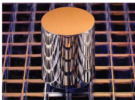
Figure 1.2 The standard platinum–iridium kilogram is kept at the International Bureau of Weights and Measures in Sèvres, France. This copy of it was assigned to the United States in 1889 and is housed at the National Institute of Standards and Technology. (Copyright Robert Rathe, National Institute of Standards and Technology)
